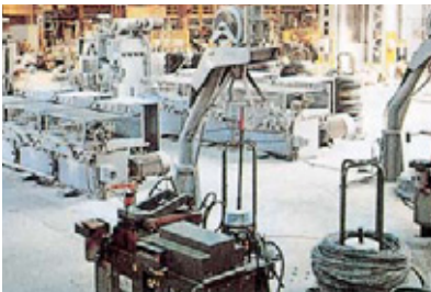
伸線機 Various wire drawing machines
